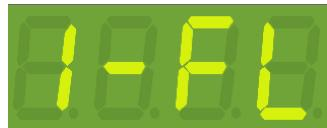
It means the first CH limit output level is FL(100%), press **【◀】** or **【▶】** to choose module 01-06 and check limit level of each channel. Module 01-06 can display level of each channel at the same time; LED of module 01 is displayed as below:
