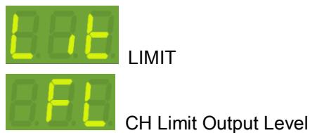
STEP-2: LD-P110 press **【ENTER】** that the channel limit output is continued blinking, and press **【▲】**, **【▼】** to choose DMX position level, and press **【ENT】** to finish editing and back to the main screen.
